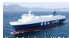
*From the Ryukyu Kaiun Co., Ltd. Website RORO ship Name of vessel: Nirai Kanai II Gross tonnage: 11,687 tons Length: 181.51 meters
